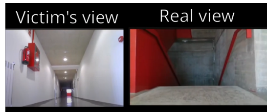
Figure 3: On the left, view of the teleoperator after being attacked. On the right, real image of the robot's situation.
