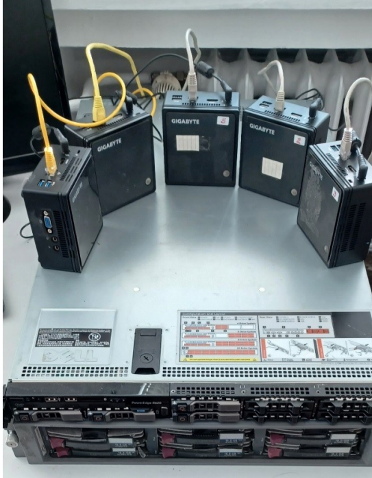
Figure 1: Cluster-based sensor network consisting of five sensor modules based on NUCs Gigabyte and control center shown in the picture below.
